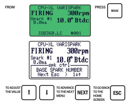
31.10 The MISC-IN SPARK NUMBER defines the spark selection number to be utilized when the Aux. Misc. Input is activated (connected to ground). The selectable range for Misc-in Spk Number is 0-8. When set to zero, this feature is disabled and will not override the active spark number.
