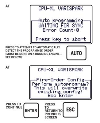
The system has the ability to attempt to automatically detect and/or verify the connections while the engine is running. **This has no effect on the engine operation.** To verify the firing order:
