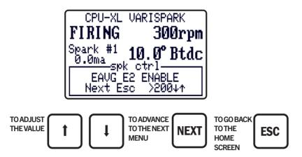
31.12 The EAVG E2 DISABLE setting determines the engine average spark diagnostic disable threshold at which the HI EAVG SPARK NUMBER selection will be de-asserted. The Enable and Disable thresholds create a hysteresis pair to add stability to the HI EAVG SPARK request function.
