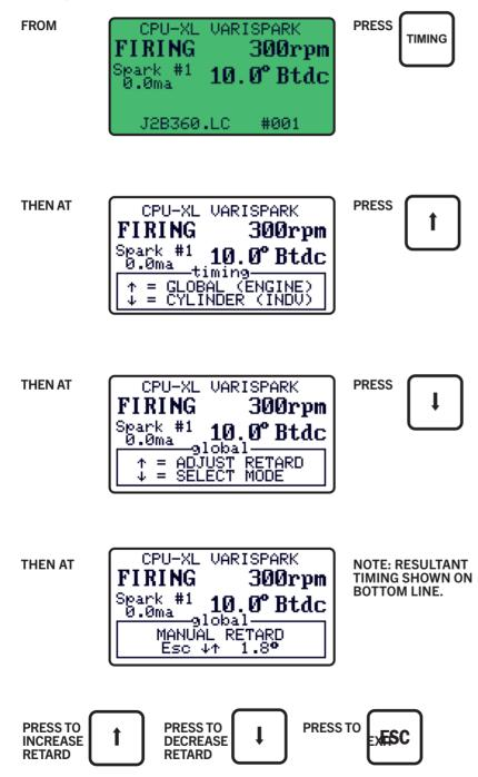
20.3 The increment of timing change is dependent on the number of holes or teeth being sensed. The minimum timing change is defined as follows.
