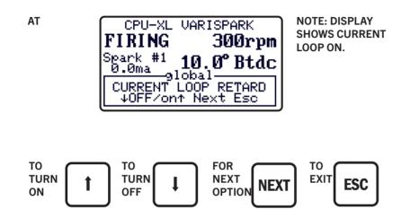
21.3 The next mode selection can enable or disable the pre-configured retard curve controlled internally by engine RPM. To configure the RPM retard curve, refer to the Programming Instructions, Form CPU-XL VariSpark PI.
