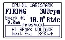
NOTE: Improper use of this feature may limit the effectiveness of the diagnostic system and result in spark reference numbers that mask real or create false problems.
