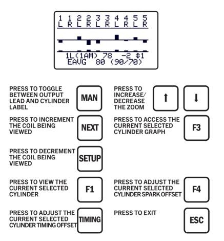
29.3 The second graph shows each individual cylinder. The solid line is the cylinder data while the dashed line is the engine average. In this picture, 105 corresponds to the spark number that is top of the graph and 65 is the bottom.
