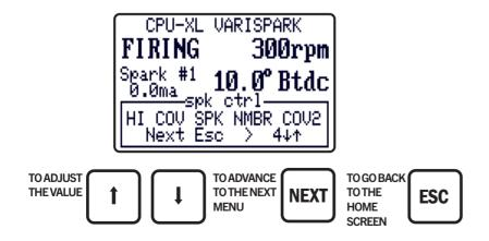
31.17 The 4-20ma SPARK MAP configuration setting enables or disables the ability to remotely control the spark number via the auxiliary 4-20mA input. When turned on, the valid 4-20mA range is limited to 2-22mA, so even when this feature turned on, the assertion of a spark number based on the 4-20mA signal will only be active if the 4-20mA signal is within the limit range of 2-22mA. If the current is outside of the range, a warning is asserted.
