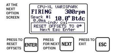
NOTE: This does not affect default settings. To zero default settings, perform this action, then perform SAVE CYL OFFSETS action (Section 23.2).
