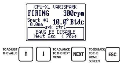
31.13 The HI EAVG SPK NMBR E2 defines the desired spark number to be asserted when the HI EAVG spark number is asserted. The range of this configuration value is 0-8 where zero disables the function entirely and 1-8 would be the desired spark selection for the special condition of high engine average diagnostic values.
