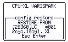
The Logic/Display Module will read the configuration from the ignition EEPROM.
