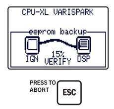
After reading and verifying, the contents are written to the eeprom of the Logic/  $\ensuremath{\mathsf{Display}}$  Module.
