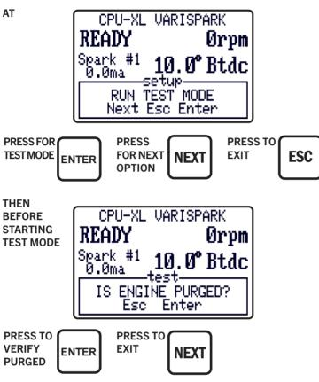
WARNING: The operator MUST fully purge the engine of combustible mix– tures prior to selecting the test mode operation. Pressing the enter key again is a confirmation of this action.
