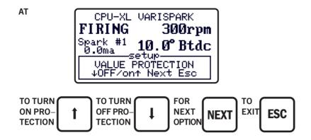
24.5 The VALUE PROTECTION can be password protected. The password PROTECTION LOCK is enabled under the programming options from the PC terminal program. See the Programming Instructions, form CPU-XL VariSpark PI for details. When password protection is enabled the following menu appears instead of the VALUE PROTECTION menu.
