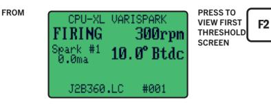
28.2 If the CAVG reference number of a cylinder is below the LO SPARK VOLTAGE threshold, a diagnostic warning for that cylinder will occur. This test will identify a low voltage demand condition which may result from a shorted coil, secondary lead or spark plug. To disable diagnostic, set value to zero.
