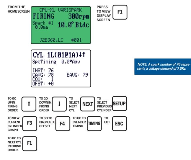
27.3 The offset adjustment screen (F4) permits the operator to adjust an offset to the spark reference number ( $\pm$  15 counts) to compensate for minor variations in reference numbers between individual coils of the same type and voltage demand.
