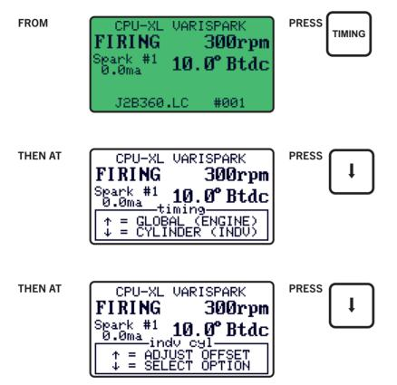
23.2 The first function is used to save the current (temporary) individual offsets to EEPROM memory. When this is done, the ignition will load these offset settings every time the engine starts or reset is pressed. Reference Section 22.3 to adjust individual offsets.
