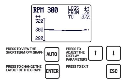
This screen shows the current running RPM as reported by the ignition system. It also shows the log range being shown. The up and down arrows to the right of "LOGS" indicates whether or not there are more valid logs before (up) or after (down) the current range.
