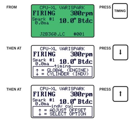
22.3 The individual timing adjustment screen identifies the primary output to be adjusted, and the degrees of offset in use for the output.
