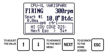
31.16 The HI COV SPK NMBR COV2 defines the desired spark number selection to be asserted when the HI COV spark number is asserted. The range of this configuration value is 0-8 where zero disables the function entirely and 1-8 would be the desired spark selection for the special condition of high COV average diagnostic values.
