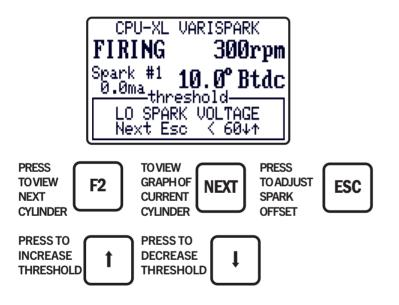
28.3 If the CAVG reference number of a cylinder is above the **HI SPARK VOLTAGE** threshold, a diagnostic warning for that cylinder will occur. This test will identify a high voltage demand condition which may result, for example, from worn spark plugs or poor air-fuel ratio control. To disable, set to 255.
