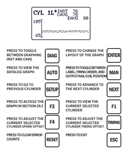
Pressing ENTER the first time will display  $\uparrow \downarrow$  and allows the user to move the graphed lines up and down using the arrow keys. This changes the spark number used for the top and bottom limits of the graph. Pressing ENTER the second time will display the  $\ddagger$  and allows the user to change the zoom level using the arrow keys. Pressing ENTER a third time exits the adjustments.
