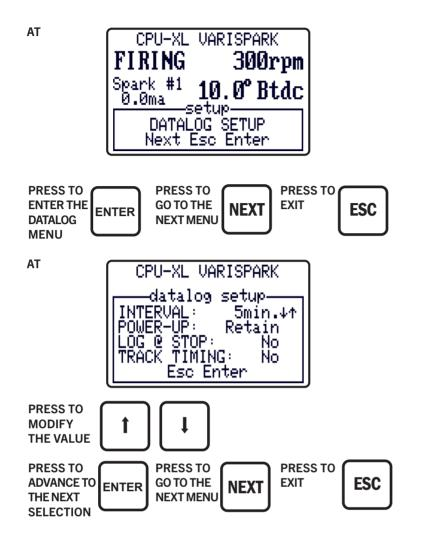
NOTE: It is possible to setup the system so that any change to the ignition timing will trigger a datalog event (an exception report). Exception reports are automatically generated for alarms or shutdowns.
