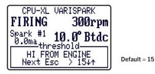
28.6 If the COV reference number is greater than the **HI VARIATION COV** threshold, a diagnostic warning for that cylinder will occur. This test will identify a cylinder whose cycle-to-cycle voltage demand has become erratic.
