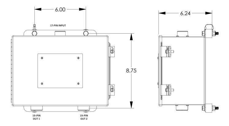
FIGURE 4: CPU-XL VARISPARK JUNCTION/DIAGNOSTIC MODULE MOUNTING DIMENSIONS
