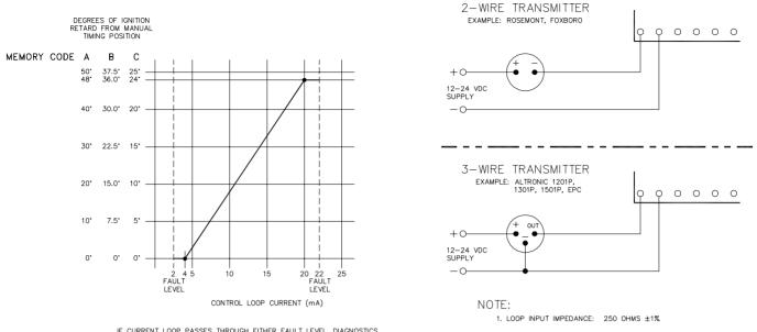
IF CURRENT LOOP PASSES THROUGH EITHER FAULT LEVEL, DIAGNOSTICS ARE ACTIVATED. - FOR STANDARD MEMORY CHIPS (.HA, .HE, .HC), TIMING GOES TO A VALUE 3 DEGREES RETARDED FROM MAXIMUM ADVANCE. - THE DEFAULT VALUE CAN BE SPECIFIED DIFFERENTLY IN A SPECIAL MEMORY CHIP (.HSXXX) OR CHANGED VIA THE SERIAL PORT USING A PC.
