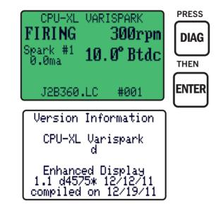
This screen displays the software build information including build number, and software version. The first screen shows the information for the display unit.
