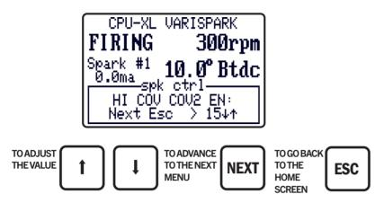
31.15 The HI COV COV2 DIS setting determines the high variation spark diagnostic disable threshold below which the latched HI COV SPARK NUMBER selection will be disabled. The coil with the highest COV is compared against this threshold. The Enable and Disable thresholds create a hysteresis pair to add stability to the HI COV SPARK request function.
