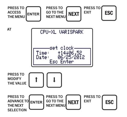
NOTE: The Logic/Display Module's real time clock does not automatically adjust for daylight savings time.
