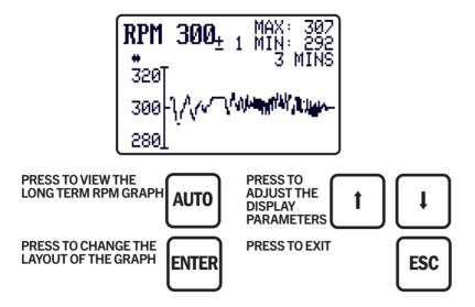
This screen shows the current running RPM as reported by the ignition system and the minimum and maximum RPM as observed over the last 5 minutes of operation. In this case, a minimum of 292 and maximum of 307 RPM were observed. It also shows the level of variation (error) that may exist between the ignition RPM and the actual RPM; in this case 1RPM. Lastly, the screen shows the timeframe being observed (1-5 minutes of operation – in this case, 3 minutes).
