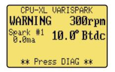
25.3 If the Alarm Out switch is being used to turn on an audible alarm or flasher, the user can acknowledge the alarm as described below.
