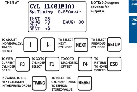
**NOTE:** In applications with narrow firing angles, the adjustment range may be limited.
