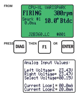
This screen displays the actual voltage values read from the Junction/Diagnostic Module as well as the current loops in both the RPM retard current loop, and spark select current loop.
