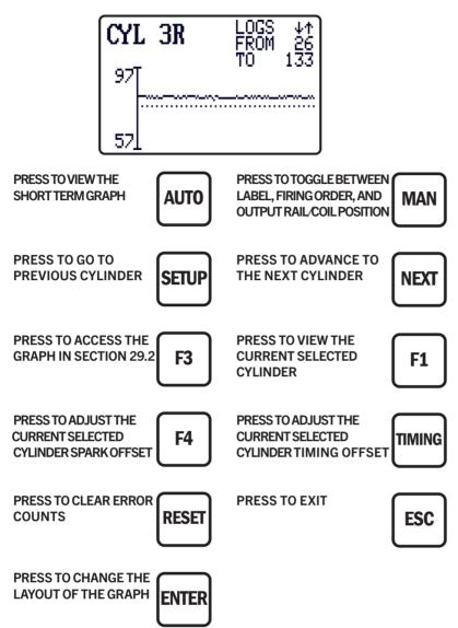
29.5 In addition to short and long term spark demand graphs, the system has a set of short and long term RPM graphs. The short term graph shows the RPM over the last 1-5 minutes to allow the operator to monitor engine speed and stability. This RPM data is what is recorded by the ignition system and should not be used in place of a tachometer or other high precision device. The RPM data is updated every 640ms during normal engine operation.
