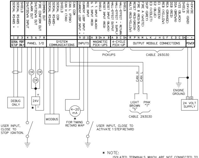
ISOLATED TERMINALS WHICH ARE NOT CONNECTED TO GROUND OR  $\pm 24$  VOLT SUPPLY. THESE TERMINALS CAN BE REFERENCED TO AN EXTERNAL ISOLATED SUPPLY IF REQUIRED.
